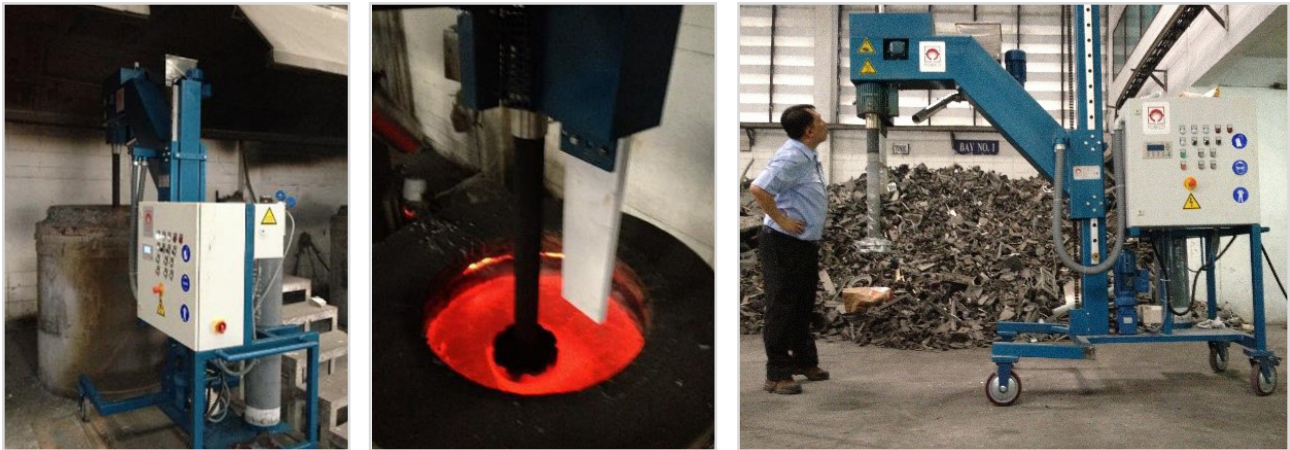
Figure 7. MTS 1500 on the fuel fired crucible furnaces used to remelt the 100% charges of A356 chips
