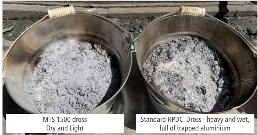
Figure 2. Dross that was collected and sampled in a very large HPDC foundry making automotive castings
