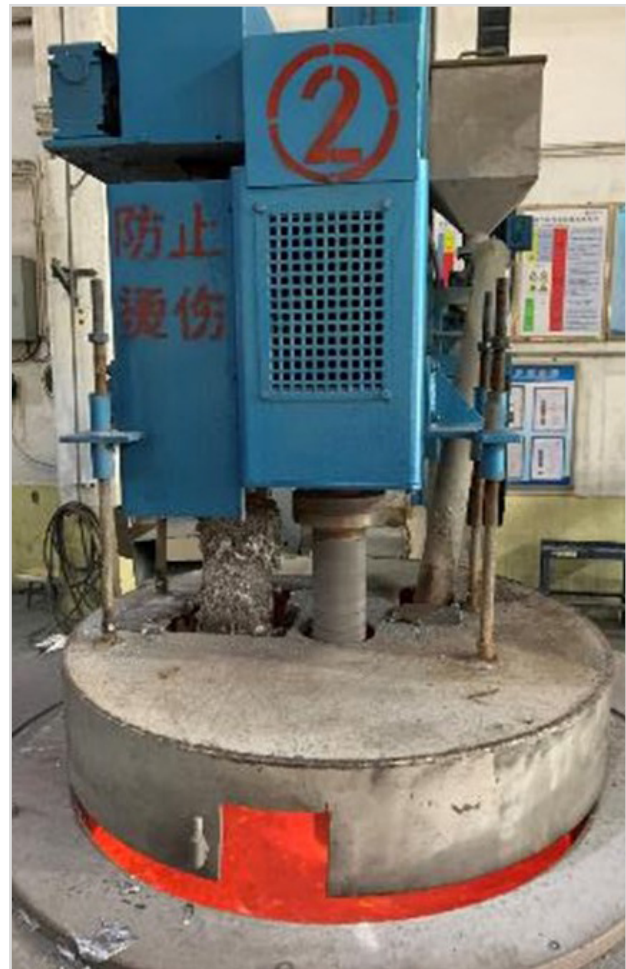
Figure 5. MTS treatment in a piston foundry
